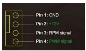
Look out for terms that may indicate the header is NOT using PWM, for example, if you see "VCC" on Pin 4 or "Speed Control" on Pin 2, then we can be sure the header does not support PWM.
